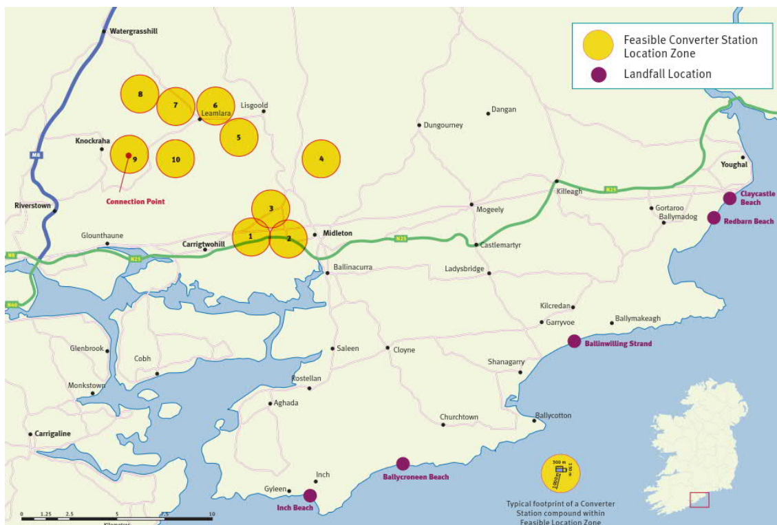
Figure 7: Feasible Converter Station Location Zones and Short List of Landfall Locations in East Cork
