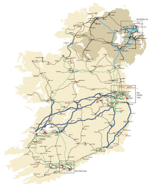
Figure 3 Heavy loaded circuits (>50%) in an intact system Winter Export
